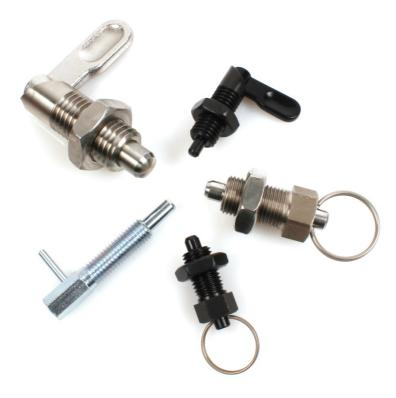
**ENGRENAGES HPC** now offers a complete range of indexing bolts. Used to block unwanted transverse movements, these index bolts are available in several versions; lockable, with a ring, lever or with horizontal fixing flange. The indexing fingers are operated by pulling a knob or by turning a lever. The ring versions are ideal for use in automated systems (for example, using a pneumatic cylinder or a remote control system).
