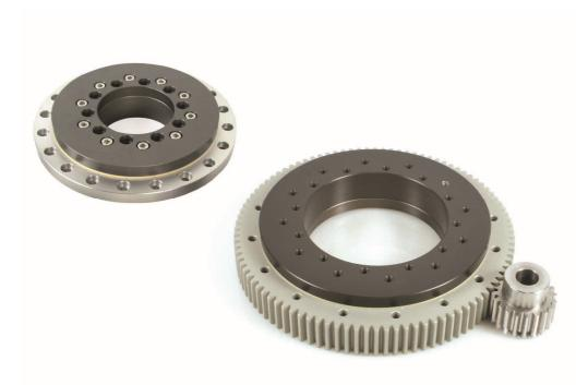
**The Engrenages HPC** catalogue includes an extensive range of rotary tables for use in conveying systems, automated machines or assembly lines. These tables are maintenance-free and have a very low coefficient of friction. Robust and easy to install, they also resist abrasion. A version with an external toothed ring can be used in combination with gears or T10, AT10 or HTD8M type pulleys.
