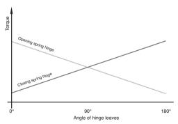
M: hinge torque at various positions M(0°): torque when hinge leaves are parallel M(90°): torque when leaves are at 90° M(180°): torque when leaves are at 180°
