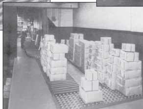
Ball transfer platform at the junction of two roller conveyors
