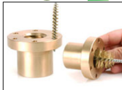
Deburring a trapezoidal nut
