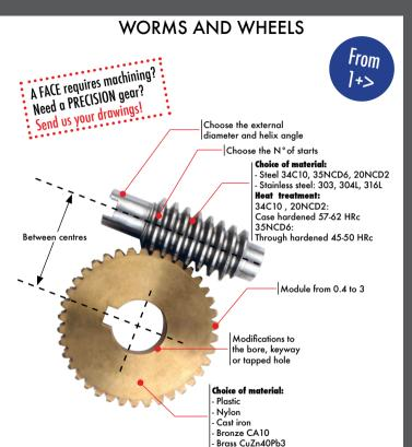
TIP: to determine the orientation of the helix angle, lay the gear flat on a table. If the teeth rise to the right, the gear has a right hand helix angle. If the teeth rise to the left, the gear has a left hand helix angle.
